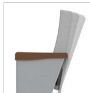
The backrest suits three-pitch positions at 15°, 18°, 21°. Seat suits at 90°
