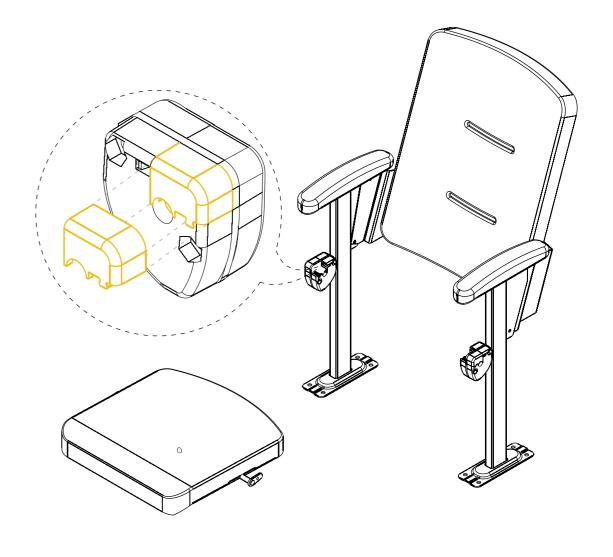
Identify the backrest according to the width of the installed legs and proceed with the assembly.
