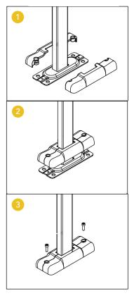
Insert the cushion shaft into support mechanism, then put the cover back on and check if it clicks.
