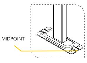
Drill holes on the floor, get the excess dust out and fix armrests using anchor bolts.
